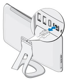
A network connection is not required to complete this computer setup, but if you have an existing network or Internet connection that uses a cable connection (such as a home cable modem or Ethernet jack), you can connect it now.
